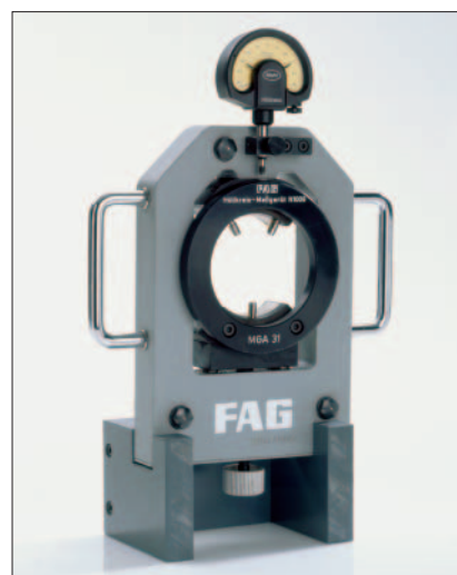
FAG enveloping circle gauge MGA 31 for setting the radial internal clearance of cylindrical roller bearings with removable outer ring
