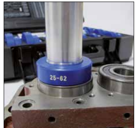
Collets are engraved and marked clearly
